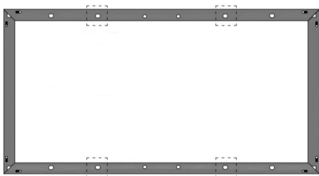
Figure 1.2 : Bolt mounting (4 mounting holes)
