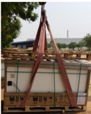
Fig: Packing Box – Adjusting Sling rope for Hoist Handling (Separator – Pallet)
